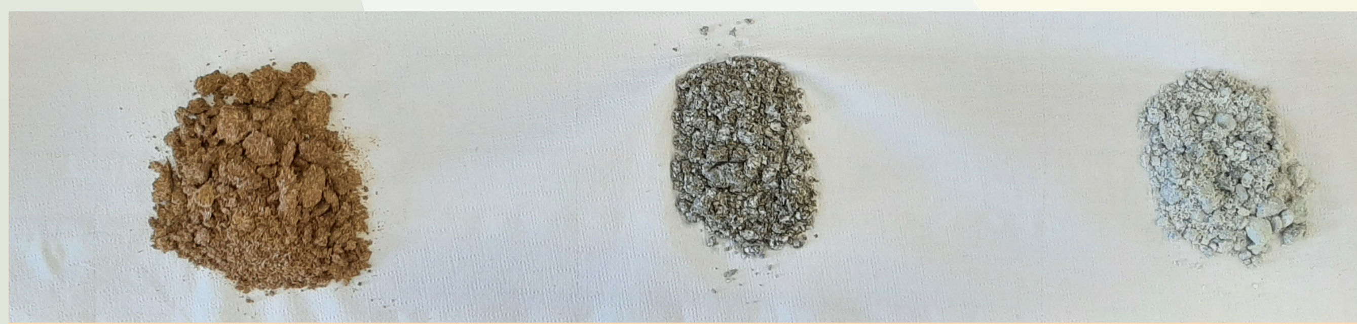
Figure 1: Samples of agro-industrial by-products. From left to right; Brewers spent grain (bio-acidification), Combination of dregs and grits (alkalinization) and grits (alkalinization)
