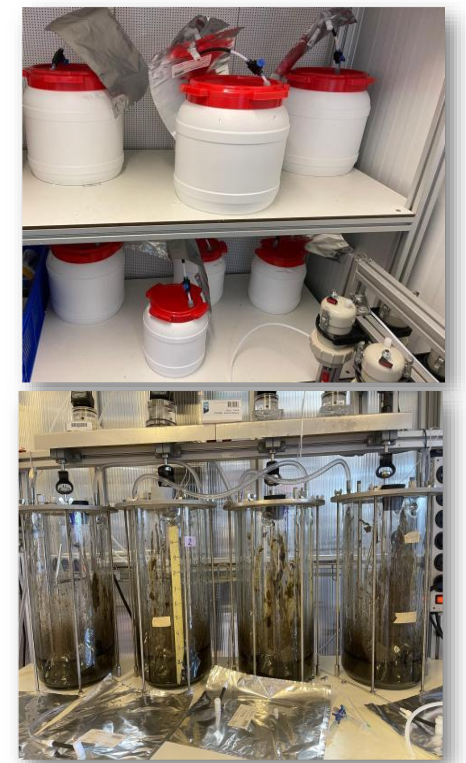
Figure 3: Anaerobic digestion reactors
